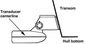
Align transducer centerline with hull bottom.
